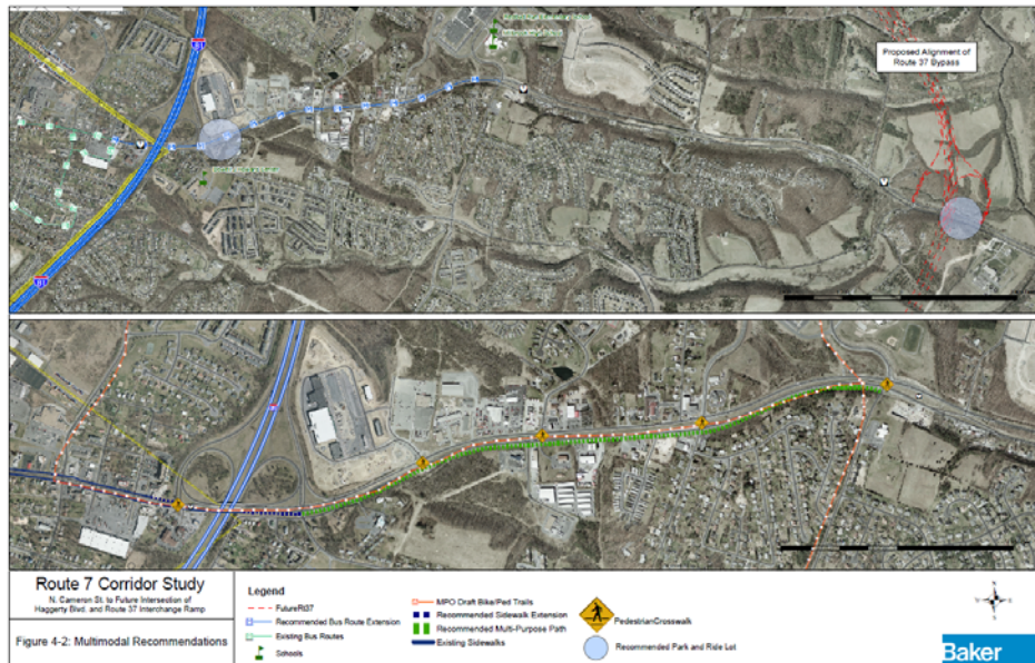
Figure 3: Overview of Recommended Multimodal Improvements
